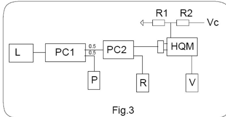
source with a fixed output optical power and an adjustable optical attenuator in series. The wavelength of the light source must be the same to that of the real system. If the HQM may operate for different wavelengths, L should generate all of wavelengths.
